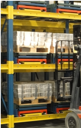
Highly efficient, expandable, pallet racking system for silver storage
